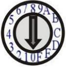
DKM01 built in rotary switch for pairing devices and the rotary switch can be used to switch 0-F channel pairing with group setting of switch 1. The channel number and group setting of the transmitter and receiver must be same to be connected each other, total up to 32 (16 for each group) pairs could be setup at one switch.
