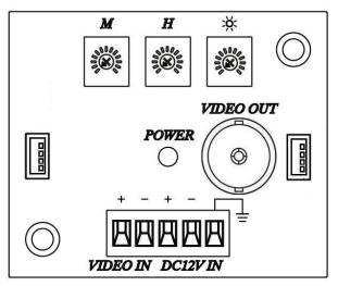
When using multi amplifier, a jumper is needed to extend power. (Max of 5 units per power adapter)
