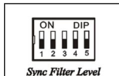
Sync Filter is designed for using UTP CAT5 cabling.
