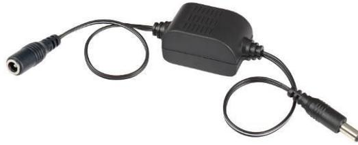
Power Ground Loop Isolator is a special designed to eliminate the video interference caused by power cable laid together with video/data cables. It could be easily install in a new or added to existing systems. It's useful where a video signal is transmitted via cable between points with different ground potentials.
