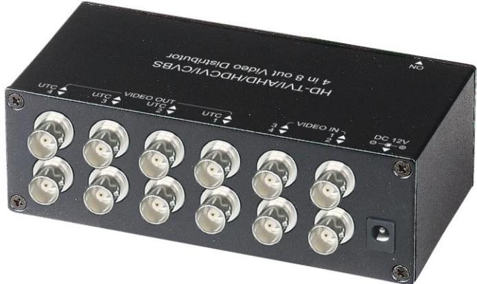
CD408HD is 4 input 8 output HD-TVI/AHD/HDCVI/CVBS Video distributor. They are suitable for far distance, different floor in a building or different electrical field.
