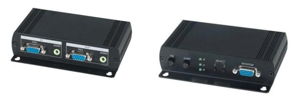
VE02ALS is designed for VGA with Stereo Audio signal over cost effective CAT5 cable to instead of VGA and Audio cable. The receiver VE02DALS receiver built in skew corrector function which could reach optimum video performance under long cable run. With chainable function allow to daisy chained another VE02DALS to extended working range over 300 meters and multiple displays.
