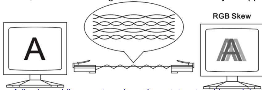
1. Recommend to use following cabling way to reduce skew status, to add special made "skew immunized adaptor", 2 pieces included at the package.
