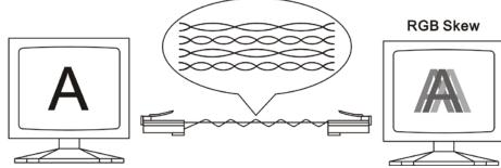
2. Recommend to use following cabling way to reduce skew status, to add special made "skew immunized adaptor", 2 pieces included at the package.
