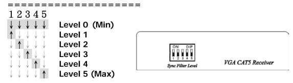
Sync Filter is designed for using UTP CAT5 cabling.
