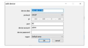
Click [Ensure] button, if the filling information is correct and the device is working normally, you will find the established device and "online" state on Device management list page.
