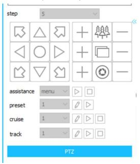
Users are allowed to control the movements of PTZ cameras in PTZ control windows, including left, right, upward and downward movements of PTZ speed doom camera; zoom in or zoom out the target, adjust focus and iris to get better image quality.
