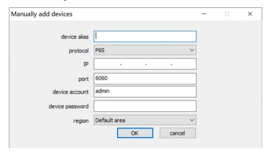
Filling in the device name, device type, device address, signal port, user name and password
