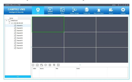
The navigation buttons on the upper line of the screen are: Real time Monitor, Remote playback, Electronic Map, Device Management, Log Query, alarm information and System Settings. Click icon to open the corresponding screen. The left part of the screen is device navigation. The right part is display area. The icon on the top right corner from the left to right are: help, logout, minimize, maximize, close. First, begin with Device Management to add devices.
