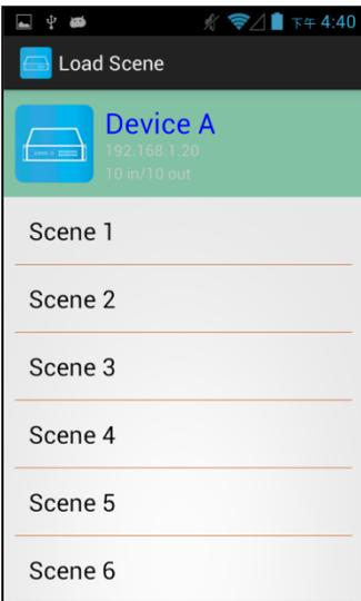
Touch scene column to load saved channels setting for all output
