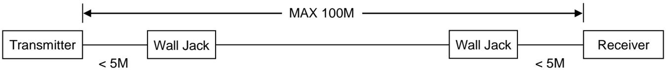
10/100Mbps network connection using general CAT5e cable and working distance up to 100M.
