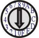
HKM02BT Transmitter built in rotary switch to set channel numbers follow 16 HEX, could switch “ 0 ~ F “ total 16 channels, A = channel 10, B = channel 11, others channel same as 16 hex conversion. For channel numbers over 15 you could use panel button, IR remote, RS-232, APP to set up.
