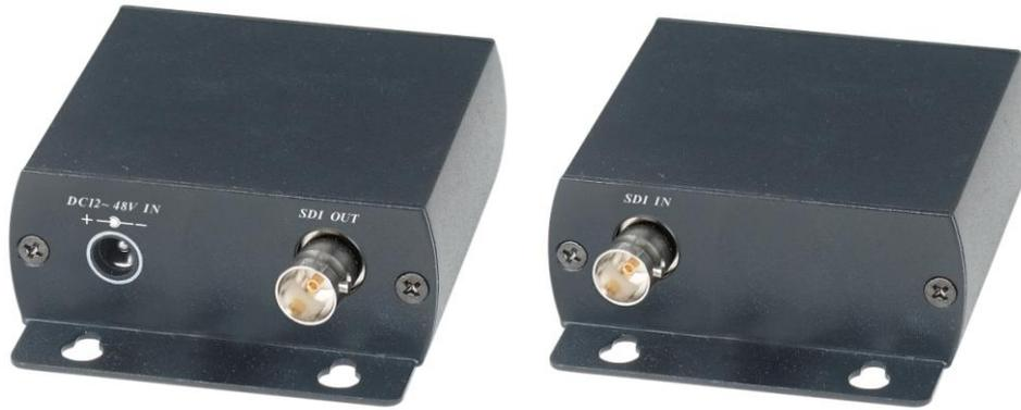
SDIVP designed is using same one coax cable to send HD-SDI video with power to HD-SDI camera. It can offer real-time and un-compressed broadcasting video quality, up to 1080p resolution and comply with SMPTE 292 , in additional, This can be used in application fields which the camera side not easy to have local power. Such as HD CCTV, machine vision, medical/equipment inspection..etc.
