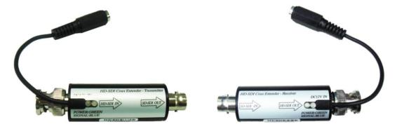
SDI06 designed is to extend the HD-SDI signal up to 300M by using  $75\Omega$  coax RG6U cable. The special feature is resolve the HD-SDI request high quality high bandwidth coax cable issue and allow to using existing old RG59 coax cable to send HD-SDI signal up to 125M when you updated the analog camera with HD-SDI Digital system.
