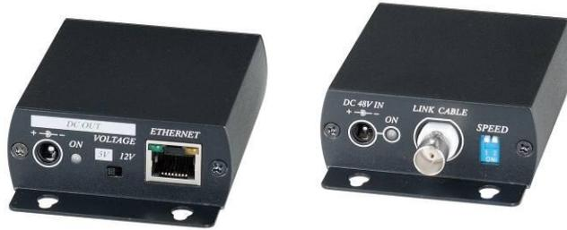
IP02EP IP extender is designed to extend any TCP/IP devices for long range transmission up to 500M over existing coaxial cable. The benefit could send power to camera use over same coax cable. It is perfect to add one IP camera with power over existing CCTV analog video camera environment. It is a great surveillance solution for sending IP video links to remote camera installation that are beyond the 100 meters distance limit of Ethernet and also provide camera power together.
