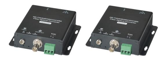
HD401F support HD-TVI/AHD/HD-CVI/HD-TVI/CVBS 4-in-1 Video signal over Fiber cable. Based on digital uncompressed HD composite video technologies which convert the AHD, HDCVI, HD-TVI or CVBS composite signals to optical signals to reach long distance up to 20KM.
