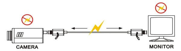
Recommend WT104PE Outdoor CAT5 UTP Twisted Pairs cable with PE jacket and steel wire, and use surge protector SP003-SP006 to avoid the damage of twisted pair system under lightning, thunderstorm weather environment.
