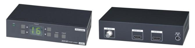
HE05CT HDMI DVB-T modulator generates a digital high definition channel from an HDMI source which can be supplied over a coaxial cable network to digital TV sets or STB's in the system. The TV required compatible with DVB-T.
