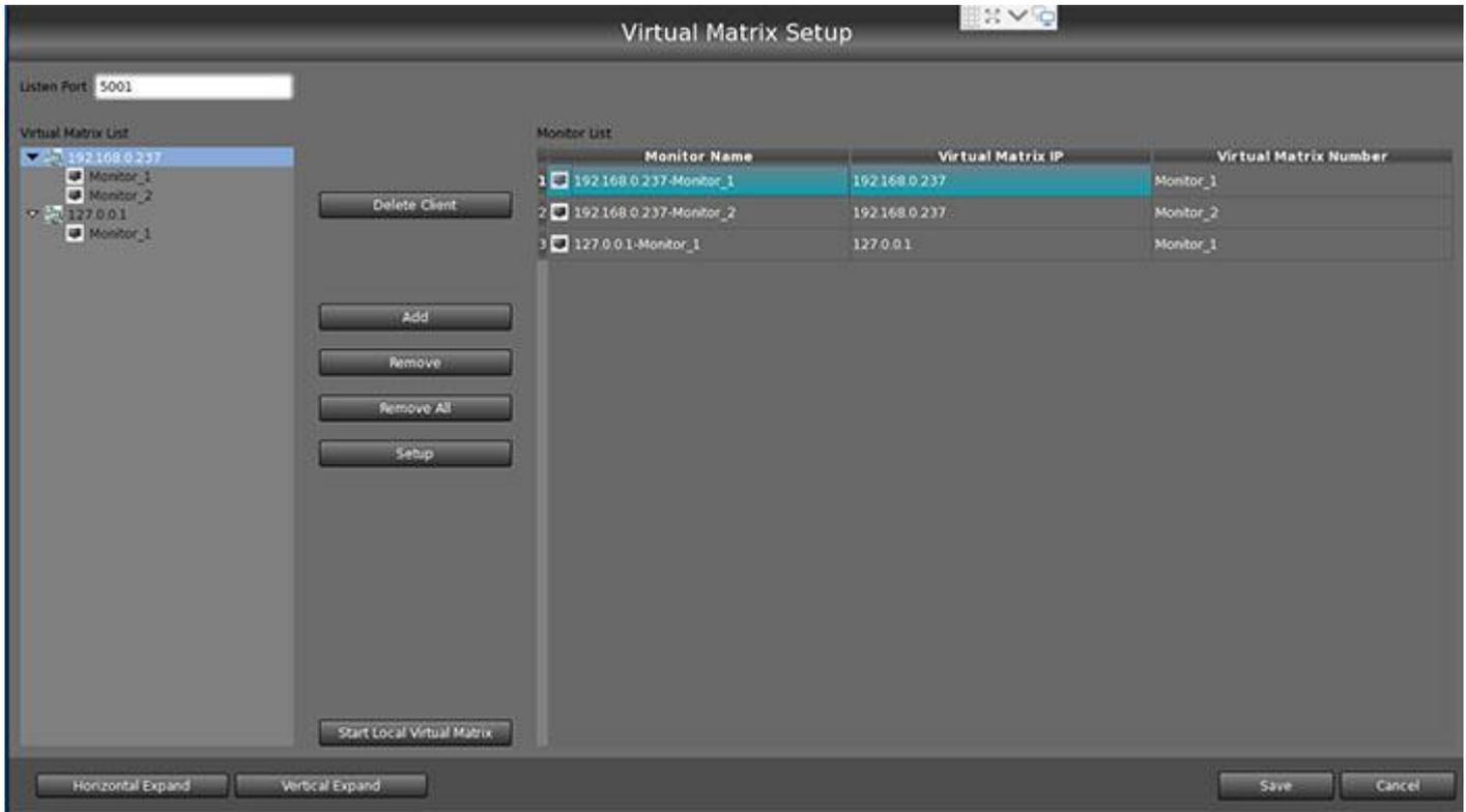
Double click the monitor of "127.0.0.1-Monitor1" to set live view for sub monitor. Main monitor supports up to 144 splits, sub monitor supports up to 16 splits.
