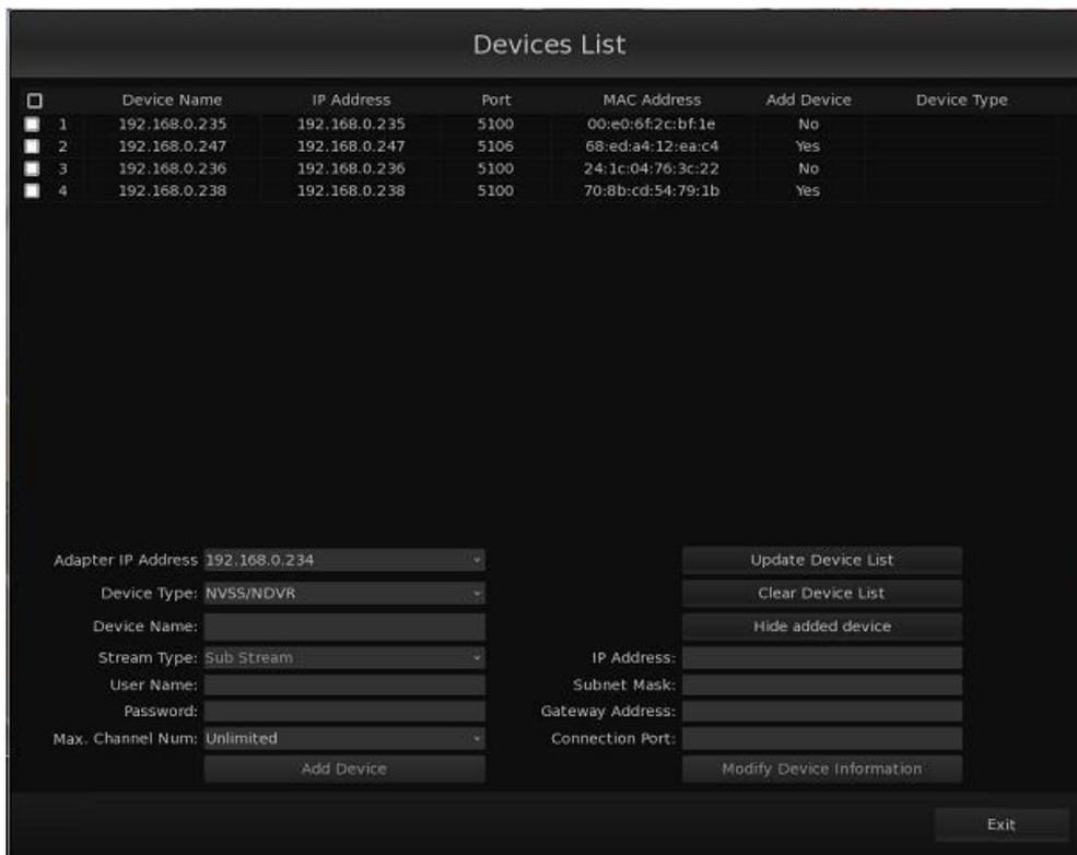
The System will display all the IP devices that are found and can be connected. You can also sequence the searched IP device by clicking the head of any column.
