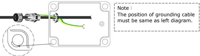
5. Through the cable <u>lock the nut</u> into the waterproof, then <u>make the RJ45 connector</u> (1) (2) (TIA / EIA-568-B), and lock the nut into the waterproof set.
