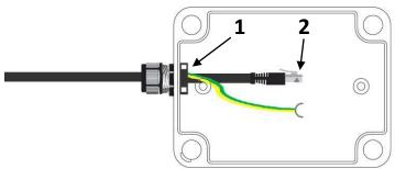
6. The other end is also <u>connected to the RJ45 connector</u>, and <u>make the nut locked</u> into the waterproof set. (1) (2)
