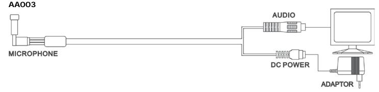
Remark: Since Hi sensitivity microphone, AA003 audio pick up box must be put at 5 meters away from monitor to avoid any audio reverberation.
