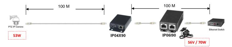
Allow to connect external power adapter when IP04X90 power is insufficient for multiple POE repeaters or long cable length application.
