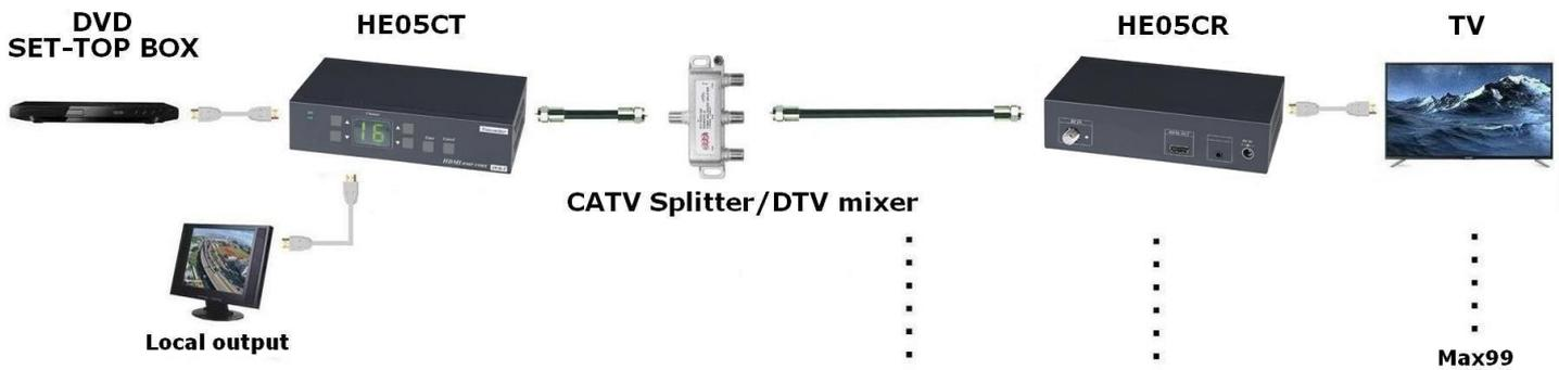
Multiple TX to multiple RX connection (with splitter)
