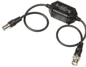
The GL001HDP Video Ground Loop Isolator is a passive devices which reduce Ground Loop Interference with HD CCTV signals and can easily install in a new or added to existing systems. It is useful where a video signal is transmitted via cable between points with different ground potentials, Differences in ground potentials are typically caused by unbalanced power line loads.
